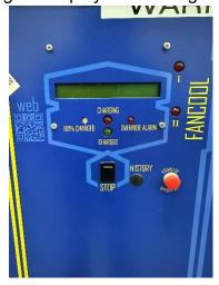
b. The image below is of a Stanbury charger when it is turned ON and is charging the battery. The charger's display does light up.
