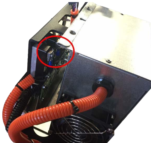
Figure 1: The charger assembly with a red circle showing the relay terminals to be avoided.
