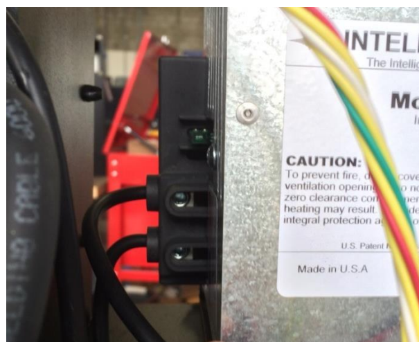
Figure 4: Charger connections. The bottom wire connects to the contactor and the top wire connects to the power inlet.
