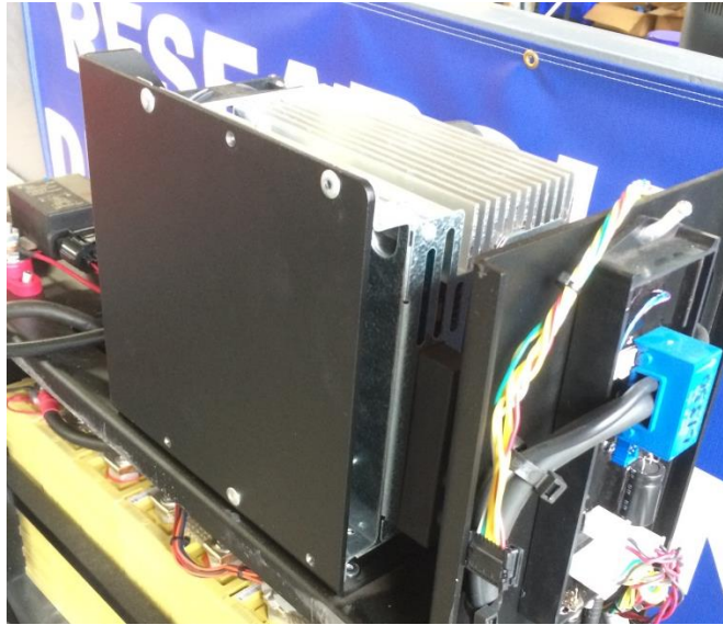
Figure 5: The charger mount and rivets.
