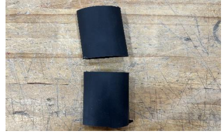
Figure 6: Cut heat shrink in sections of 1.5 in
