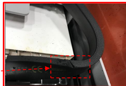
Figure 4: Right most positive busbar
