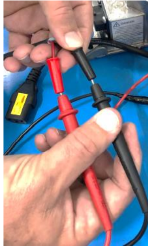
Figure 6: Connecting voltmeter to prototype jumper
