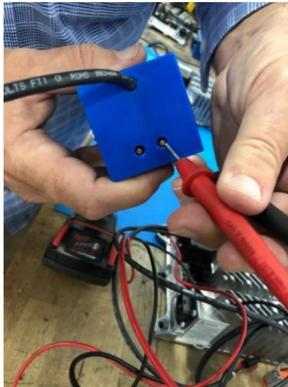
Figure 11: Connecting voltmeter to prototype jumper
