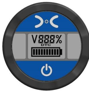
Figure 2: The BDI and its capacitive touch button.
