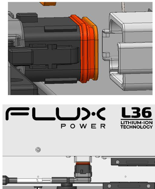
Telematics harness connection is a 4-pin connection:
