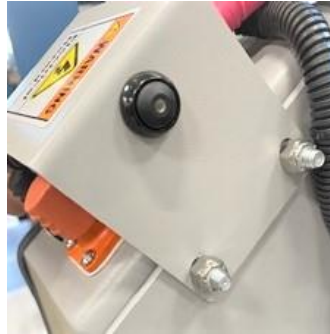
Figure 2: On/Off Push Button located on top of Power Cables. Hold down to activate the battery.
